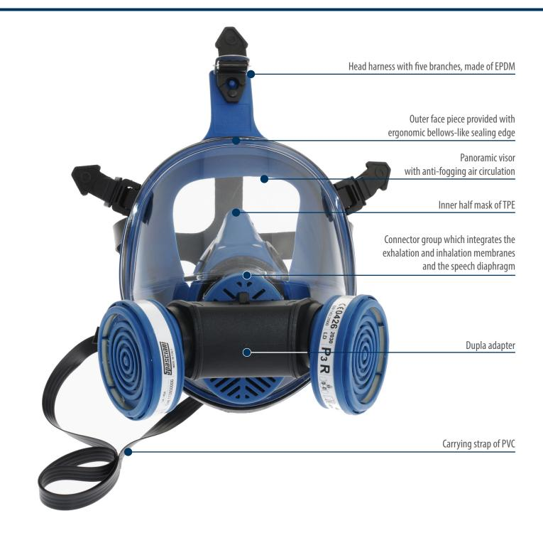
**DUPLA** is a negative pressure full face mask with threaded connector to EN148-1. DUPLA integrates a panoramic visor and can be used both with screw filters to EN 148-1 and special cartridges of the Spasciani 2000 series.
